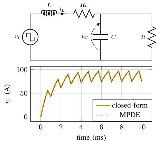
**Fig. 1:** Simplified circuit of the buck converter in continuous conduction mode (top) and solution calculated with the new basis functions compared with the closed-form solution (bottom).
