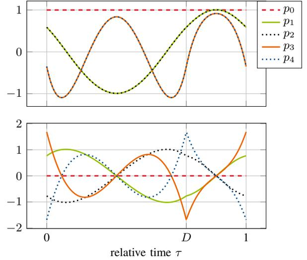
**Fig. 3:** Transformed PWM basis functions  $g_k(\tau)$ ,  $k \in \{0, 1, 2, 3, 4\}$ , i.e.,  $N_p = 4$ . (top) real part. (bottom) imaginary part.
